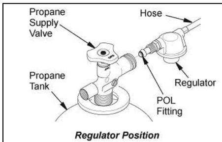
3. Connect the hose to the valve inlet connector. Tighten firmly using a wrench.
